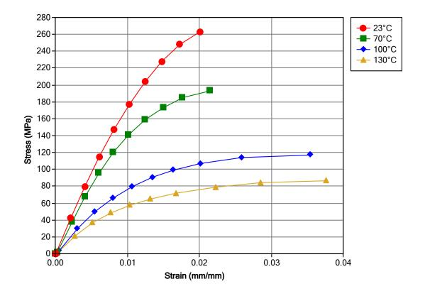
Secant Modulus vs. Strain (ISO 11403)
